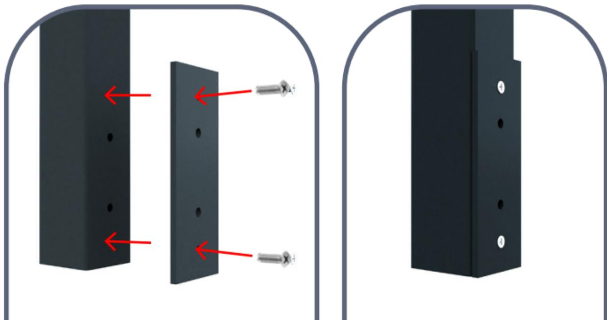
**Attach the metal plate on the post using the pre-drilled hole as a guide.**
